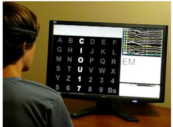
Fig. 1. Example of a P300 Type Spelling BCI using a 6X6 Matrix of Letters and Numbers, and a Backspace[17]
